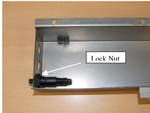
6. Install the new igniter and secure it with the lock nut. The nut should be snug, but do not over tighten.
