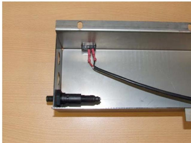
9. Carefully lower the control panel cover over the two knobs. You may have to reconnect the igniter wire if it is too short to reach up over the knobs.
