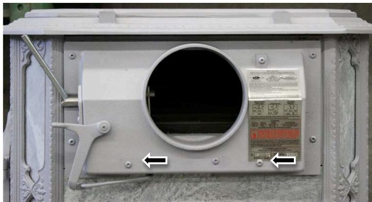
3. Insert the bolts provided through the rear heat shield, through the spacers, and thread them into the holes in the flue collar. If you are installing an outside air adapter, use the middle button head bolt to secure the right tab of the adapter to the stove first. Pass the left bolt through the shield, spacer, left tab for the adapter, and then thread it into the flue collar. Tighten with the 7/16" wrench.
