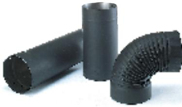
Stovepipe comes in 6", 7", and 8" diameters, in lengths of 12", 18", 24", 36", and 48". There are 90° elbows (fixed and adjustable), a 90° tee with cap, 45° elbows (fixed only), several slip/adjustable lengths, and a variety of diameter adapters. Each pipe comes with a set of 4 screws for a securing connections. Stovepipe can be painted to match the cast iron color of your stove.
