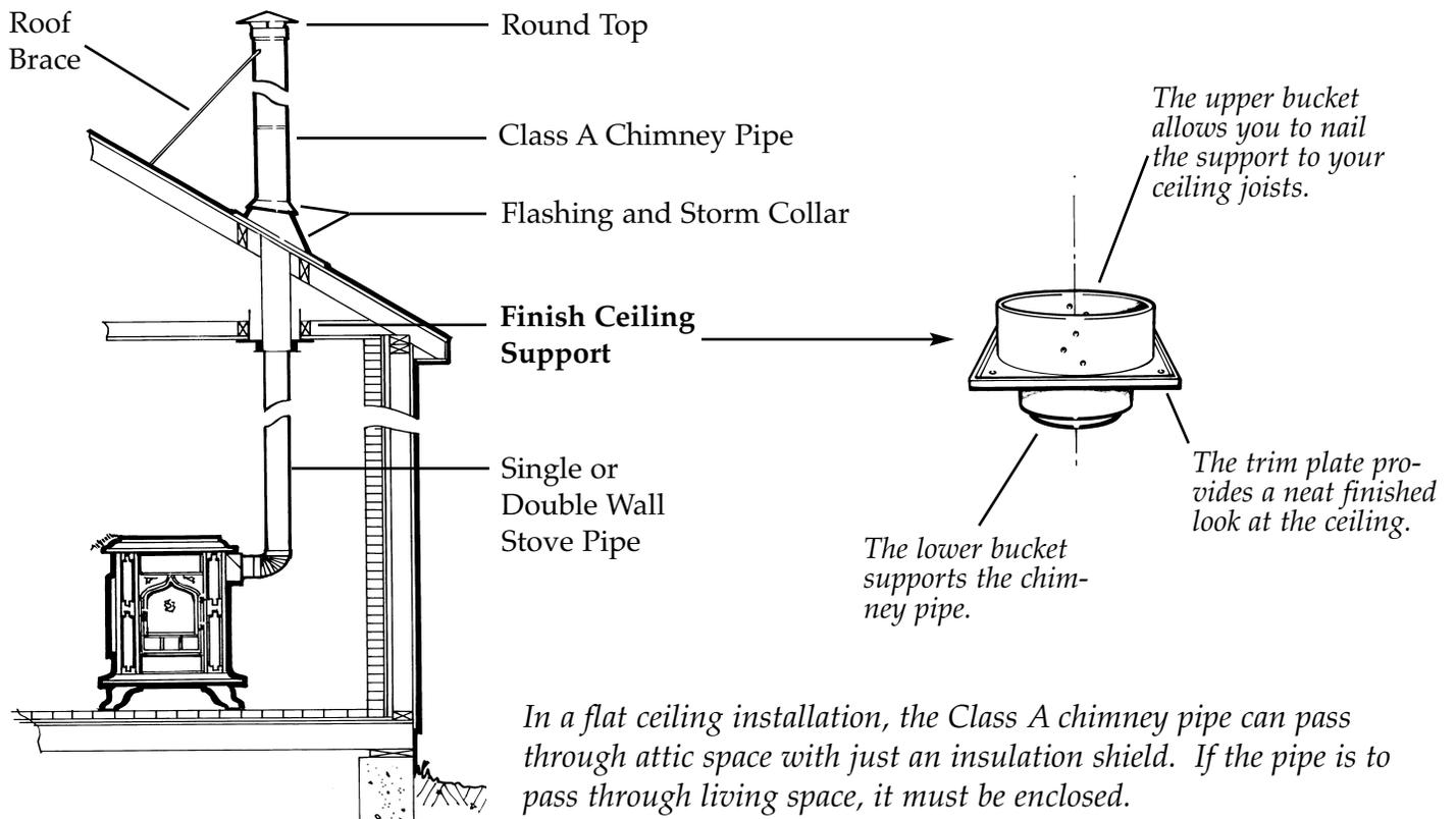
Installing a chimney in a room with a flat ceiling is quite straightforward. Your stovepipe will start at the stove's flue collar and go up to the ceiling. The Finish Ceiling Support will be installed in the ceiling to provide the necessary clearance and structural support for up to fifty feet of chimney pipe.
