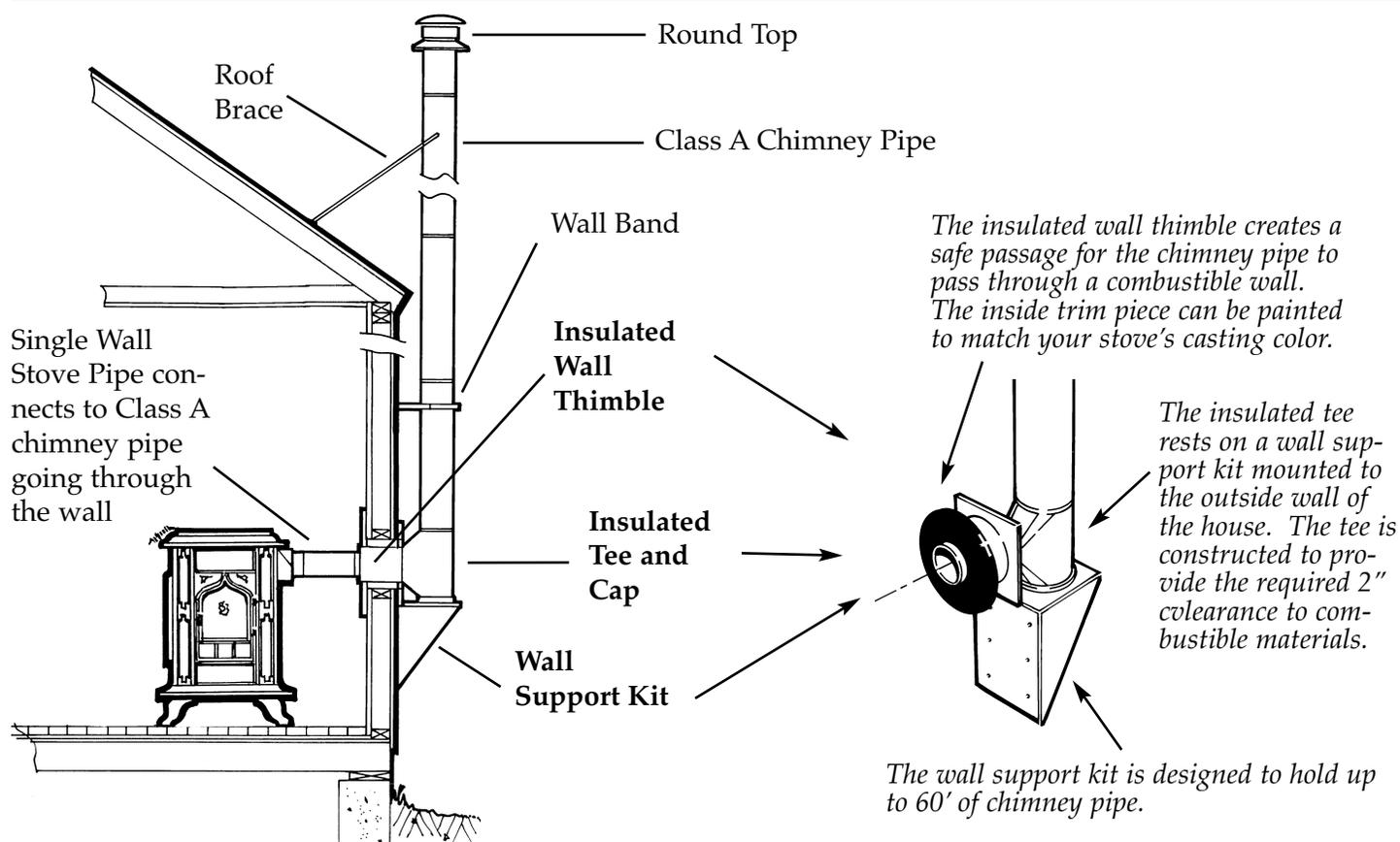
If your stove location requires your chimney to pass through an exterior wall and run vertically up the side of the house, Metalbestos has a kit to get you through the wall safely. While the Metalbestos system is completely safe to “stand alone” we would highly recommend building an insulated chase around the pipe on the outside of the house to help keep it warm. This will help promote good chimney performance and reduce creosote formation. (See “What makes a good chimney”).
