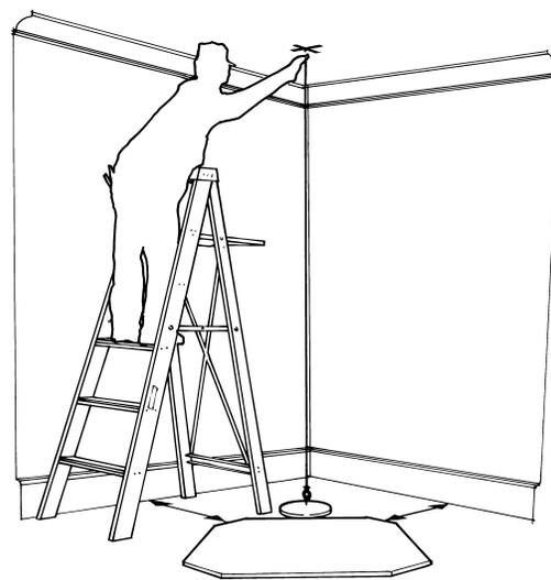
"lay out" your installation and make sure pipe will be straight and plumb.
