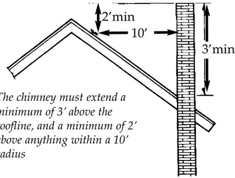
This is where knowing your roof pitch comes in. Roof pitch is the number of inches the roof rises vertically for every twelve inches it runs horizontally. It is expressed as inches of rise/inches of run, such as 3/12, 4/12, 5/12. To figure out how much pipe you will need above your roof line, multiply the rise or numerator of your roof pitch (3 or 4 or 5, etc.) times ten and add 24 inches. This is the total number of inches of pipe you will need above where you penetrate the roof.
