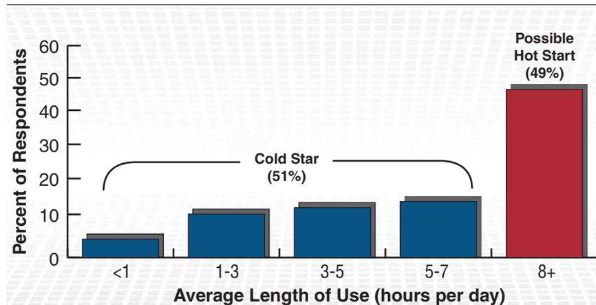
Catalysts in wood heaters reach operational temperature (approximately 550°F) within 10 to 20 minutes of start of fire in contrast to longer times needed for secondary combustion to control air emissions from non-catalytic heaters. An HPBA consumer survey showed that more than half of home wood heater events probably began with cold starts from the fact that 51 percent had an average use period of less than seven hours (plenty of time for the heater to cool down).
