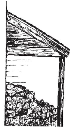
*Wood can be stored and stacked in a variety of structures both simple and complex. The key to success is to keep the wood dry, exposed to as much sunlight as possible, and to stack it in a way which allows air to circulate freely around it.*
